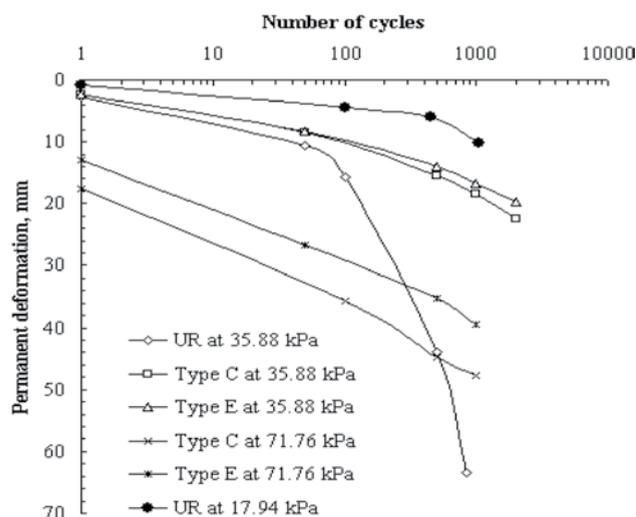
Fig. 7 Permanent vertical deformations versus number of load repetitions behaviour of different models
