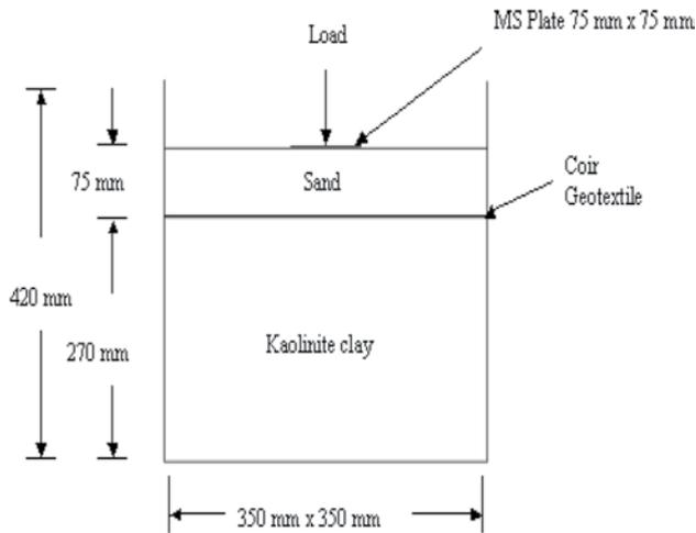
Fig. 5 : Schematic sketch of experimental setup
