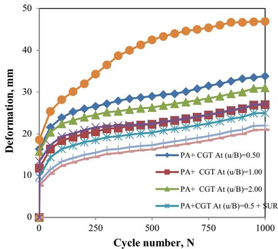
Fig. 15 : Cyclic deformation versus number of cycles for CGT reinforced pond ash
