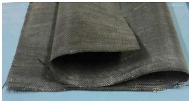
Fig. 8 : A view of the woven geotextile (WGT)
