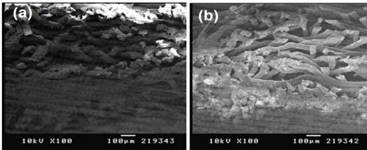
**Fig. 6 :** Cross sectional view of used nonwoven media (a) without nanofiber (b) with nanofiber
