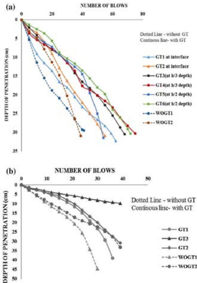
**Fig. 22 :** a Variation of penetration with number of blows for Road 5. b Variation of penetration with number of blows for Road 7
