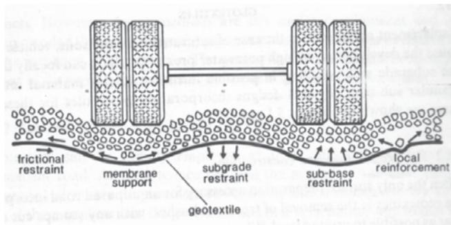
**Fig. 1 :** Geotextile stabilization of an unpaved road
