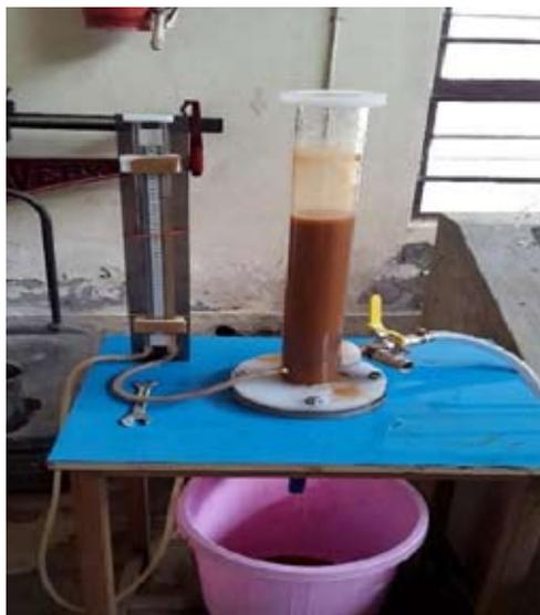
Fig. 1 : Falling head water permeability tester
