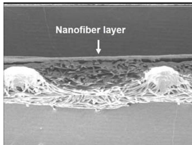
Fig. 3 : Cross section of the PVD filter jacket
