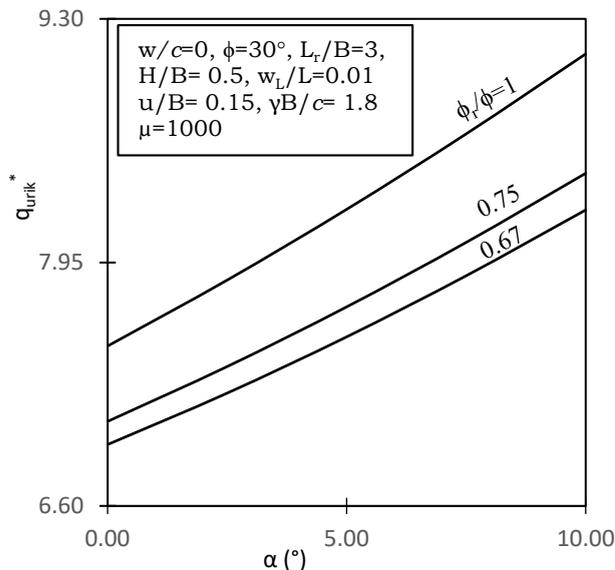
Fig. 10 :  $q_{urik}^*$  versus  $\alpha(^{\circ})$  Effect of angle interface shear resistance
