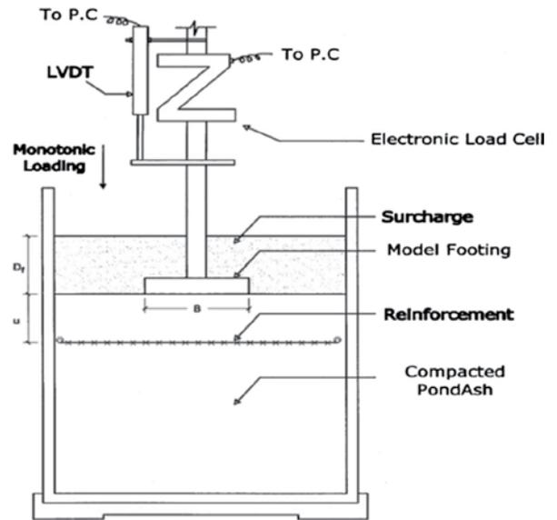
Fig. 11 : Definition sketch of the test procedure
