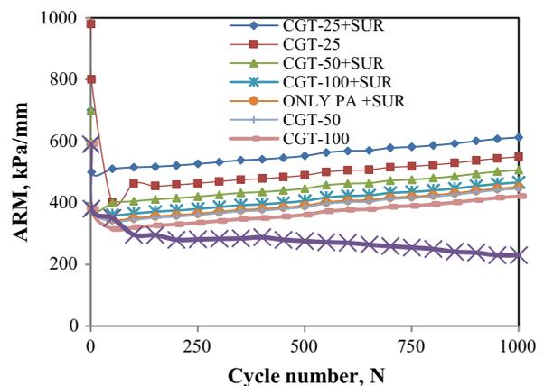
Fig. 17 : Variation of ARM with cycle number for pond ash reinforced with CGT
