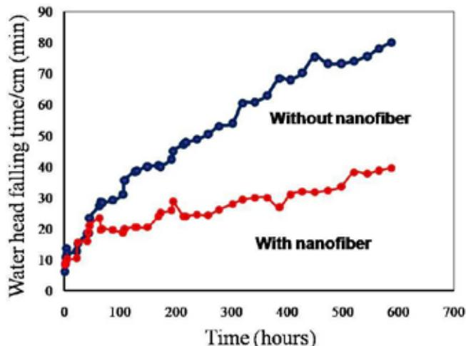
Fig. 5 : Water head falling time after continuous use in presence of soil
