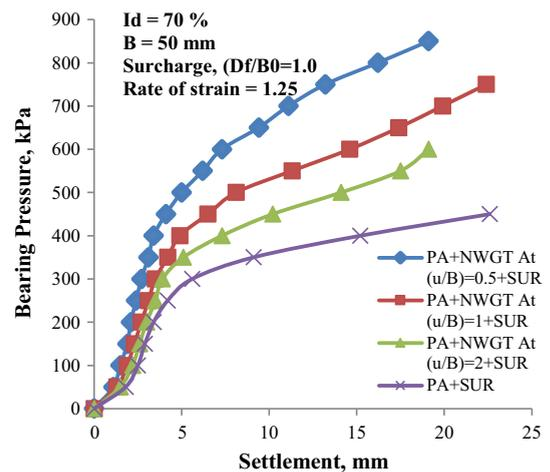
Fig. 12 : Variation of bearing pressure with settlement for WGT
