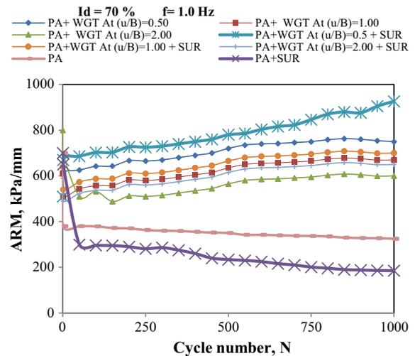
Fig. 16 : Variation of ARM with cycle number for pond ash reinforced with WGT
