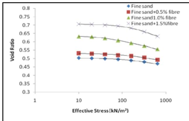
**Fig. 1 :** Void ratio-effective stress plots of unreinforced and 6mm length fibre reinforced fine sand in soaked condition
