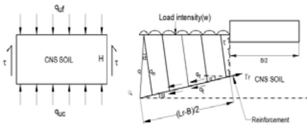
**Fig. 2 :** Stresses on soil column and inclined reinforcement
