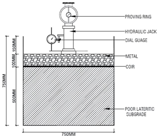
Fig. 18 : Schematic diagram of experimental setup
