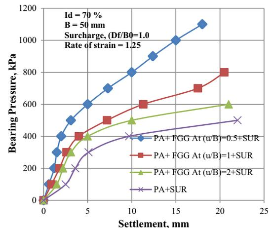
Fig. 13 : Variation of bearing pressure with settlement with coir geotextile (CGT)
