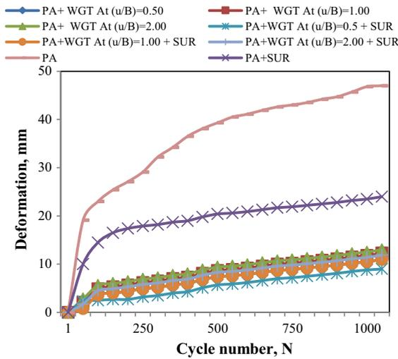
Fig. 14 : Cyclic deformation versus cycle number plot for WGT reinforced pond ash
