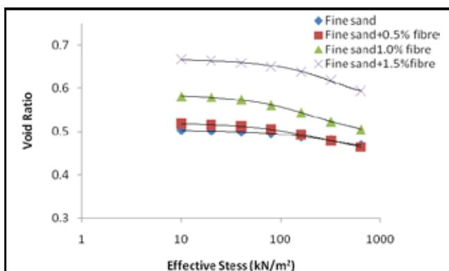
**Fig. 2 :** Void ratio-effective stress plots of unreinforced and 12 mm length fibre reinforced fine sand in soaked condition
