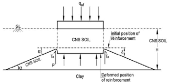
**Fig. 3 :** Additional stress developed in the inclined reinforcement due to transverse force
