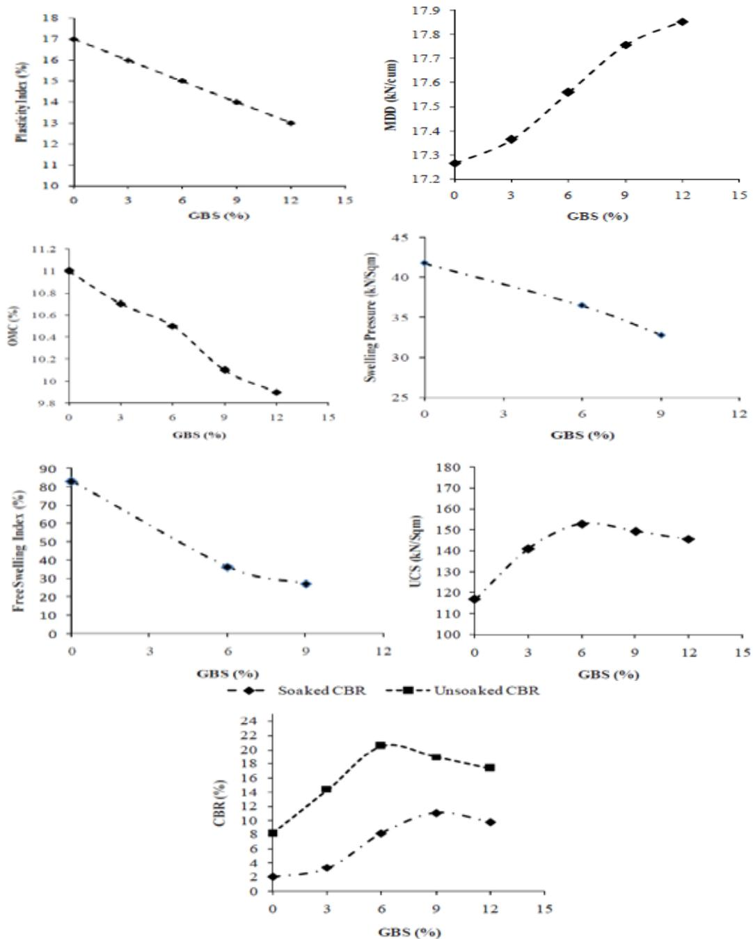
Fig. No. 8 : Comparison of physical and strength properties of soft soil mixed GGBS (Yadu & Tripathi, (2013)
