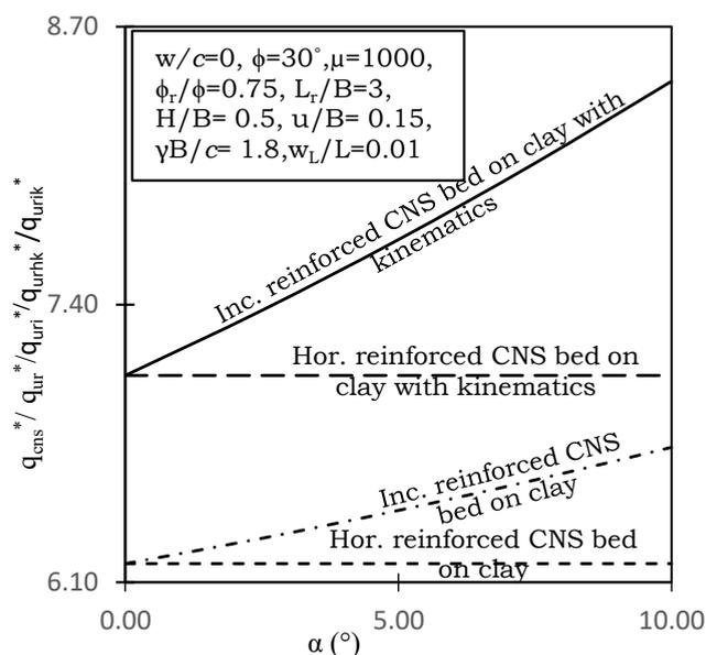
Fig. 6 : Variation of Normalised bearing capacities versus inclination of reinforcement  $\alpha$ -Effect of various techniques
