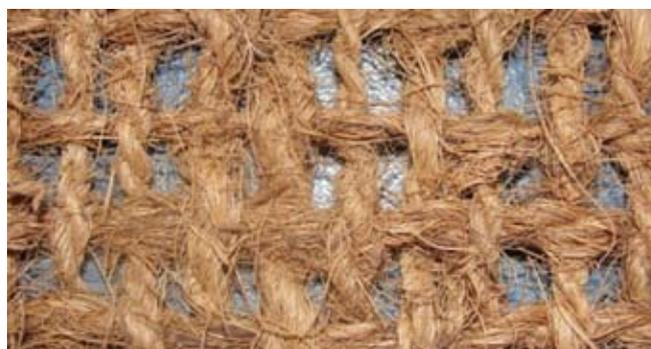
Fig. 9 : A view of the coir geotextile (CGT)
