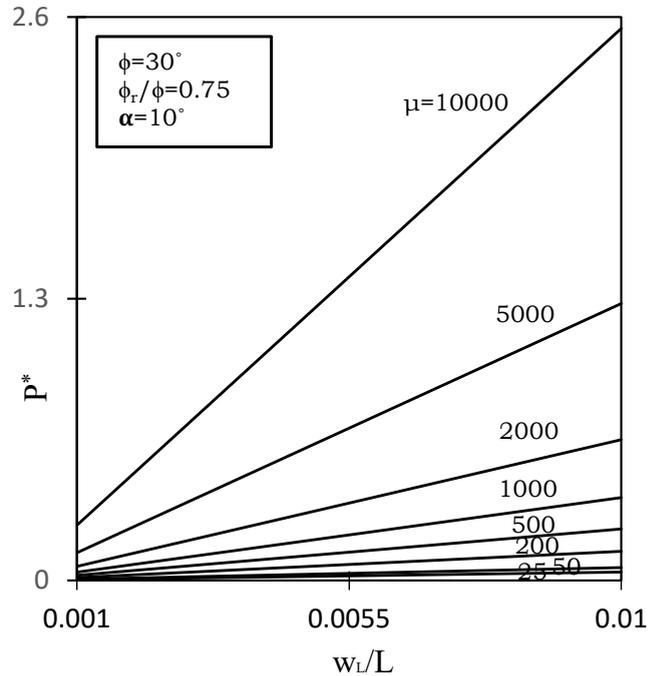
**Fig. 5 :** Variation of normalised transverse force,  $P^*$  with normalised displacement,  $(W_L/L)$ - Effect of stiffness of soil. (Umashankar and Madhav, 2003).
