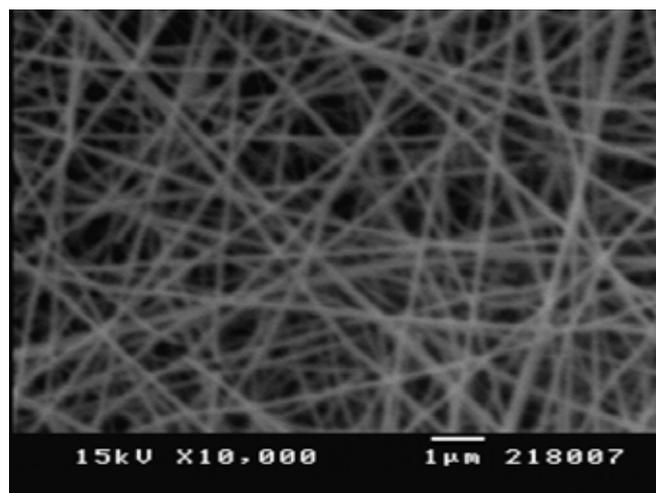
Fig. 2 : SEM image of Nylon 6 nanofiber at standardized parameters
