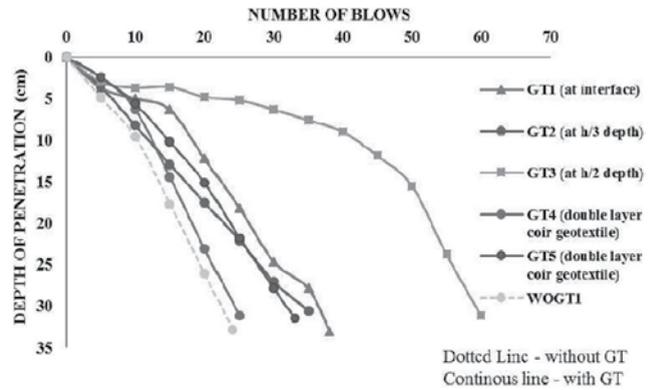
**Fig. 23 :** Variation of penetration with number of blows for Road 8
