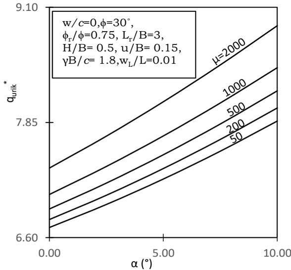
Fig. 7 : Variation of normalised bearing capacity,  $q_{urik}^*$  versus inclination of reinforcement -Effect of Relative stiffness ( $\mu$ )
