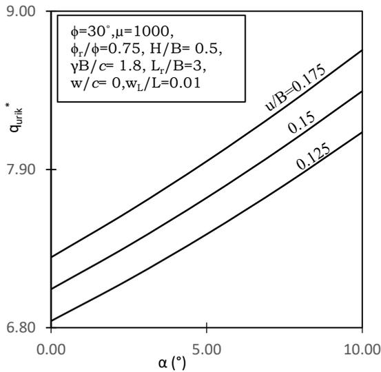
Fig. 13 : Variation of  $q_{urik}^*$  versus  $\alpha$  -Effect of  $u/B$
