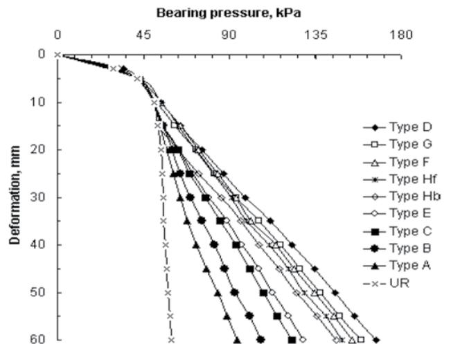
Fig. 6 : Variation of deformation with bearing pressure of all types
