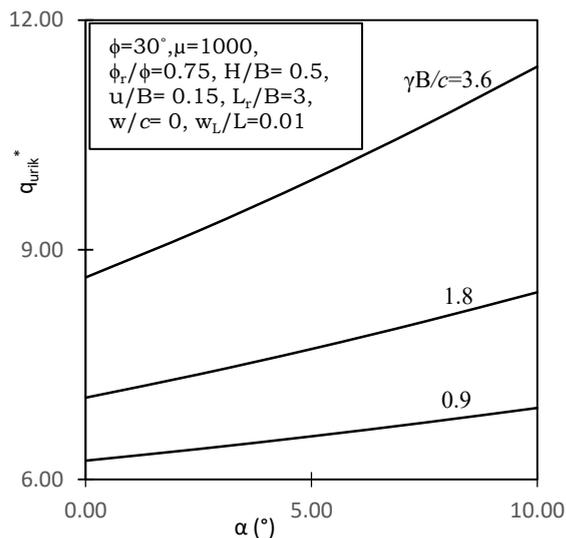
Fig. 12 : Variation of Normalised bearing capacity,  $q_{urik}^*$  versus Inclination of reinforcement  $\alpha$  -Effect of  $\gamma B/c$
