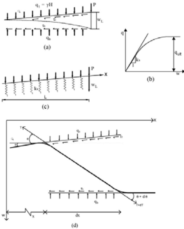
**Fig. 4 :** (a) Deformed profile (b) normal stress-displacement response of soil (c) Idealization of soil (d) Forces acting on infinitesimal element
