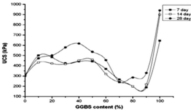
Fig. 5 : Unconfined compressive strength test with GGBS content for different curing period (Sharma & Sivapullaiah, 2011)
