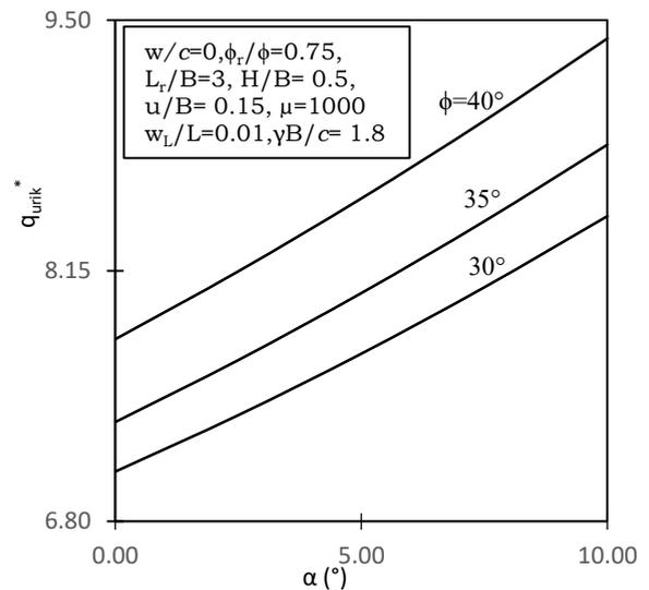
Fig. 9 : Variation of  $q_{urik}^*$  versus Inclination of reinforcement  $\alpha$ -Effect of  $\phi$ .
