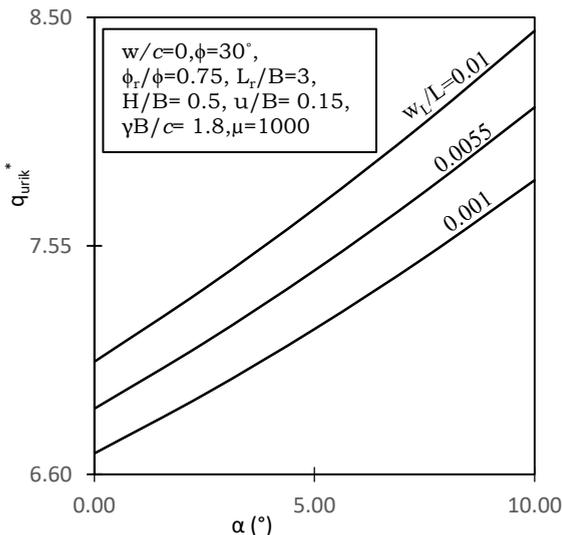
Fig. 8 : Variation of  $q_{urik}^*$  versus inclination of reinforcement,  $\alpha$ -Effect of  $w_L/L$
